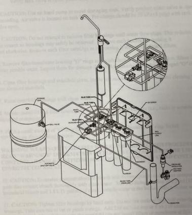
Diagram shows an air gap faucet installation,
